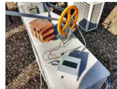
Picture 2: Atria LOC in a Junction Box w/LCD Screen Driving a Small Parabolic Trough Simulator
