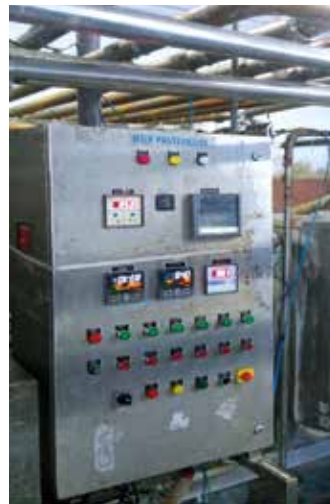
Picture 2: Milk Pasteurizer Machine; Capacity: 20,000 litres/hour; Steam Requirement: 250 to 300 kg/hour
