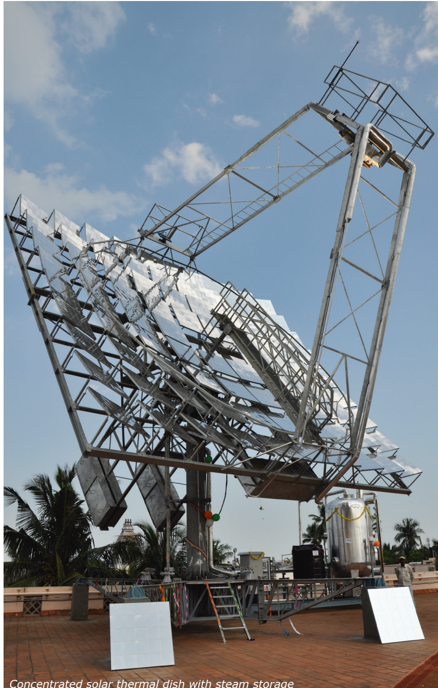
Concentrated solar thermal dish with steam storage
