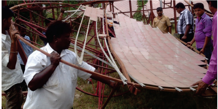
Mirror degradation observed in Scheffler concentrator
