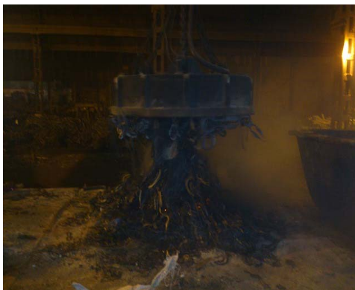
Figure 10: Overfilling of furnace
