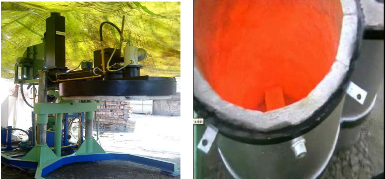
Figure 8: Ladle preheating system
