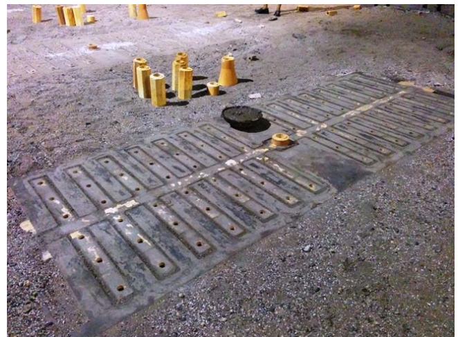
Figure 4: Runner and gate system
