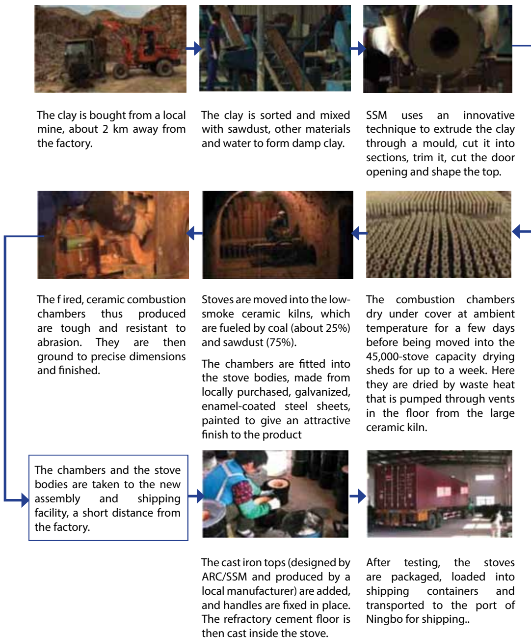
Figure 2 Production flow chart for Stovetec stoves in Shengzhou, China
