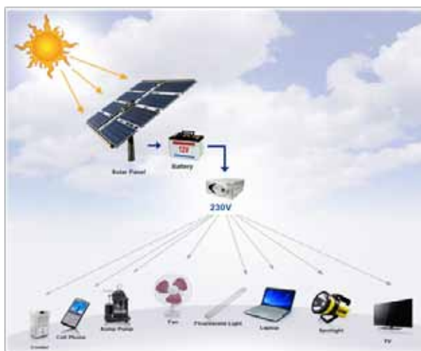
Figure 5 Schematic of solar home system Source. www.jjsolar.in
