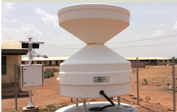
An automated rain gauge located at Bunkpurugu in the Northern Region provided by the CREW project
