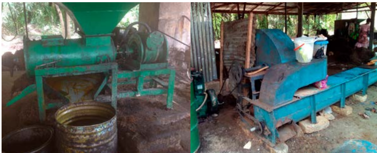
Typical example of oil mill/expeller in APO facility (left) A blower machine in an APO facility (right)
