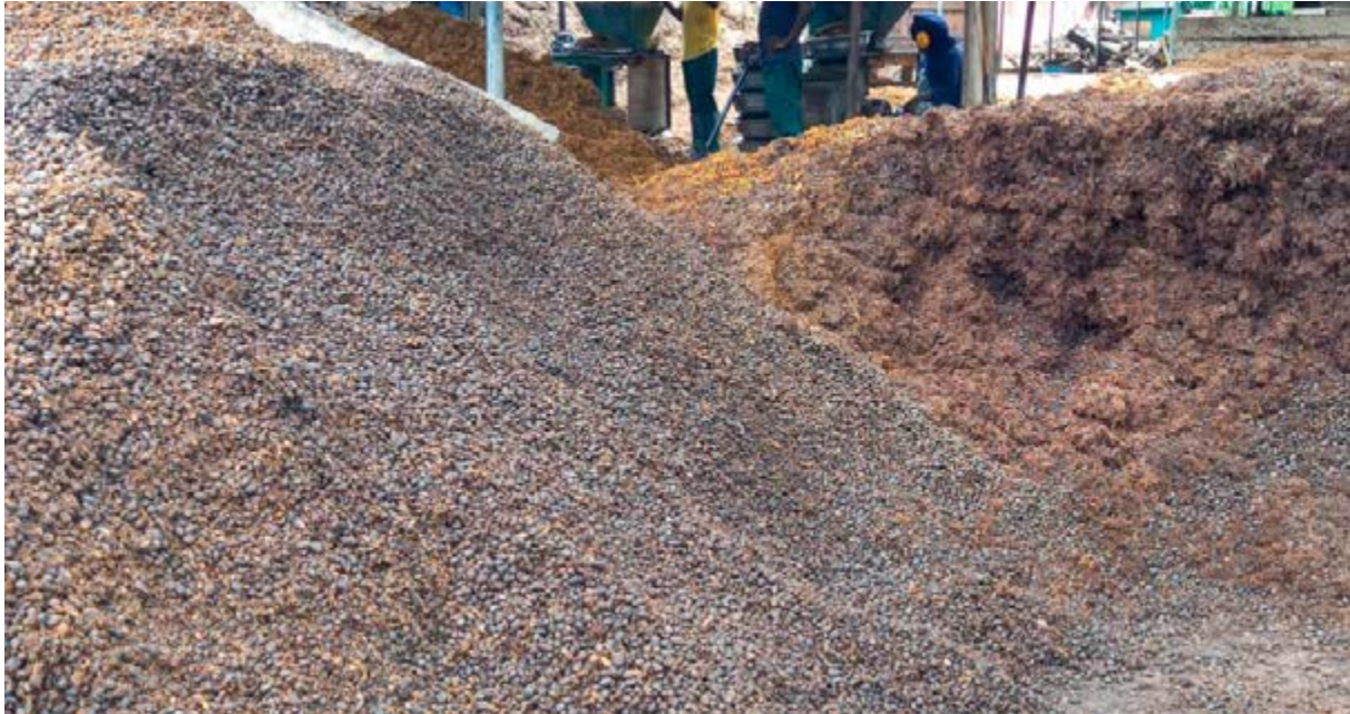
Biomass stored for use as fuel inputs into boilers
