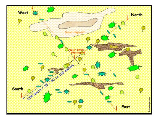
Field lay-out of the Line Intercept Measurement (LIM), Gintzburger et al. 2005 – reprinted 2009)
