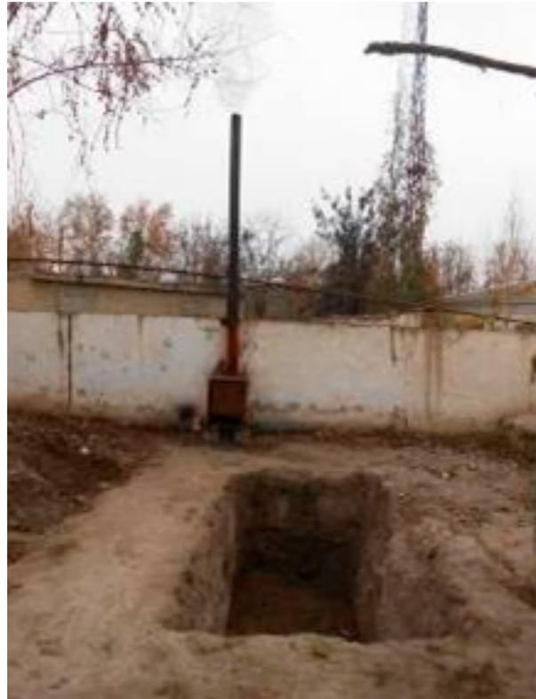
*Small scale incinerator and ash pit*
