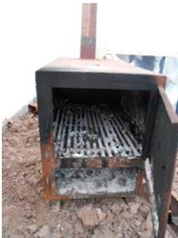
*Burning chamber of the incinerator*
