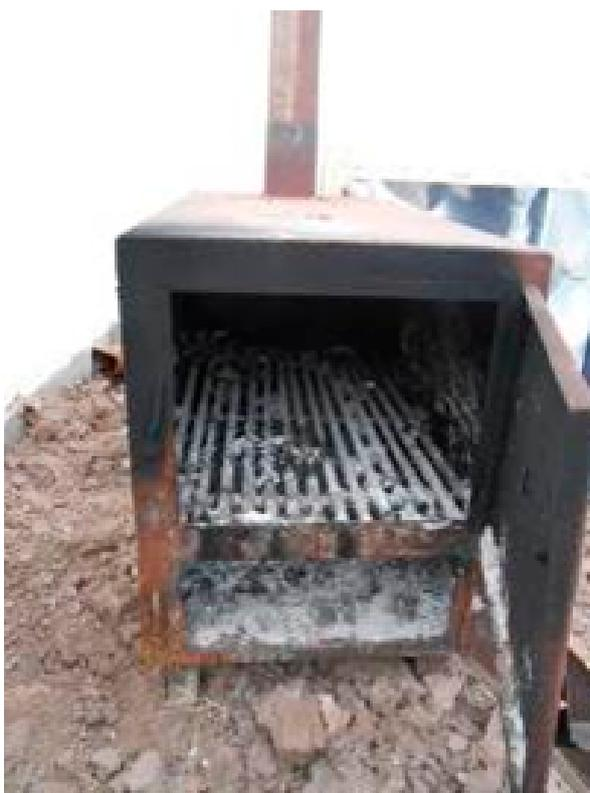
*Burning chamber of the incinerator*
