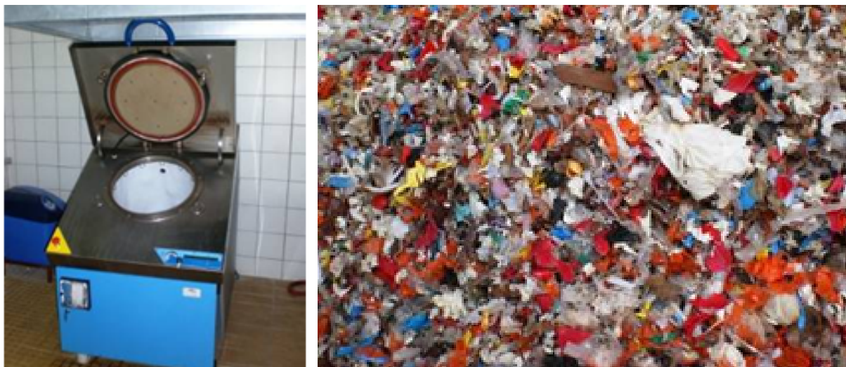
Bio-hazardous waste treatment facility at the Clinical Centre Sarajevo: Disinfection equipment (left), shredded waste after disinfection (right)
