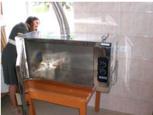
On-site microwave waste treatment system, Minsk
