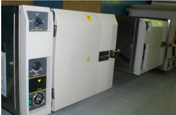
Autoclaves for waste and reused sharp containers, TB dispensary, Minsk
