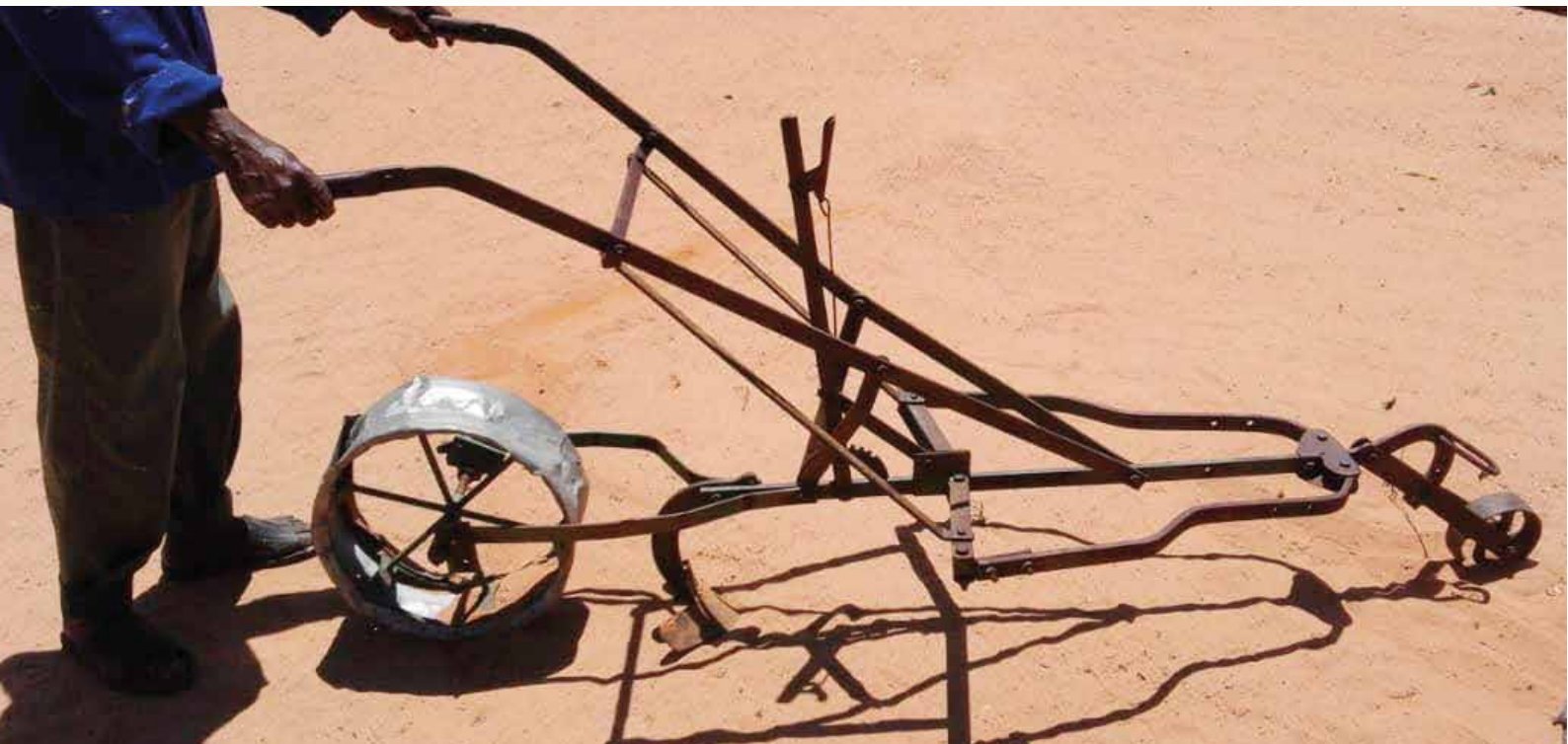
Mr. Ditau with the ripper fashioned from an old mold board plough
