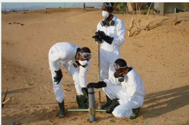
Mauritania. Technicians collect soil samples in Letfetar to assess the level and distribution of pesticide contamination as part of the country's compliance with the 2001 Stockholm Convention on Persistent Organic Pollutants.
