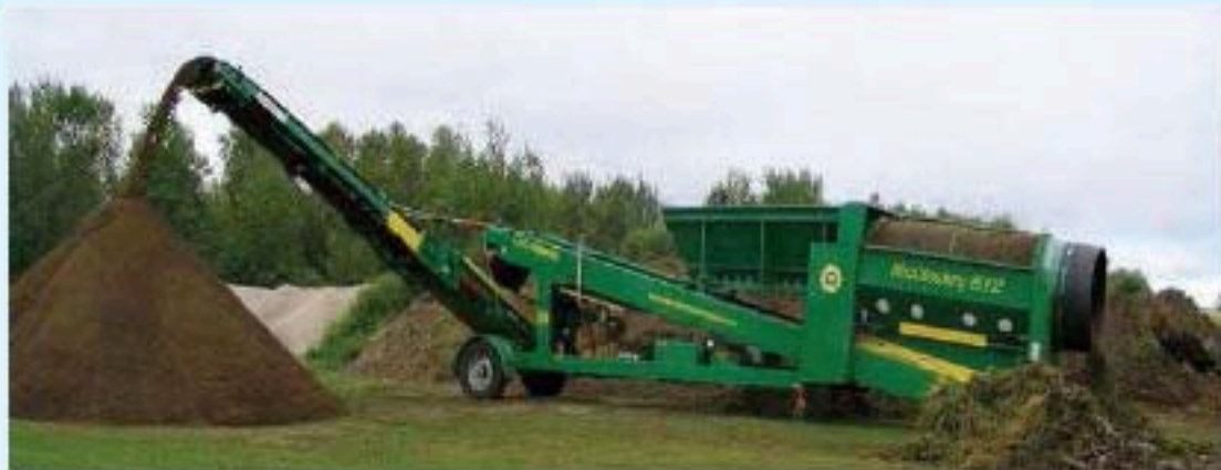
Figure 58 - Separation step (drum sieve) - Source (Mc Clostoy)
