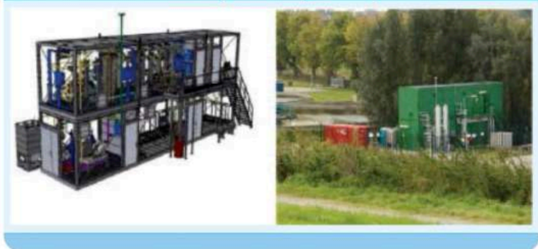
Figure 56 : Biogas treatment and liquefaction unit - Source (GPP @ 4T system - GIS)
