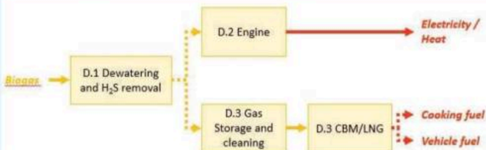
Figure 51 : Flow chart - Gas cleaning and valorization
