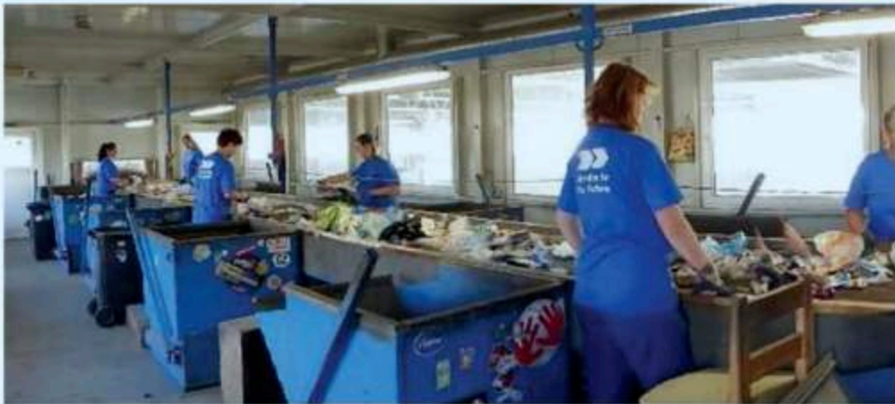
Figure 42 : Manual sorting (FCC Environment CE) Automatic aeraulic separator
