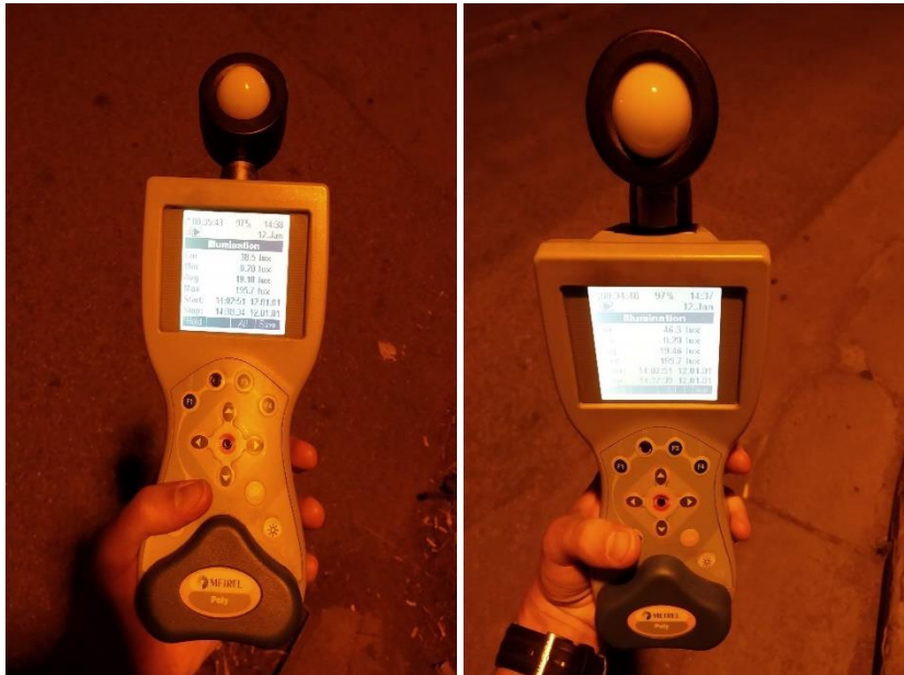
Image 41: Horizontal luminosity intensity measurement (left) and vertical luminosity intensity measurement (right)
