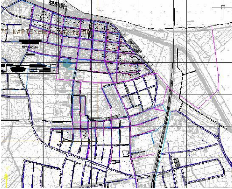
Figure 5.5 Example of Water Supply Network
