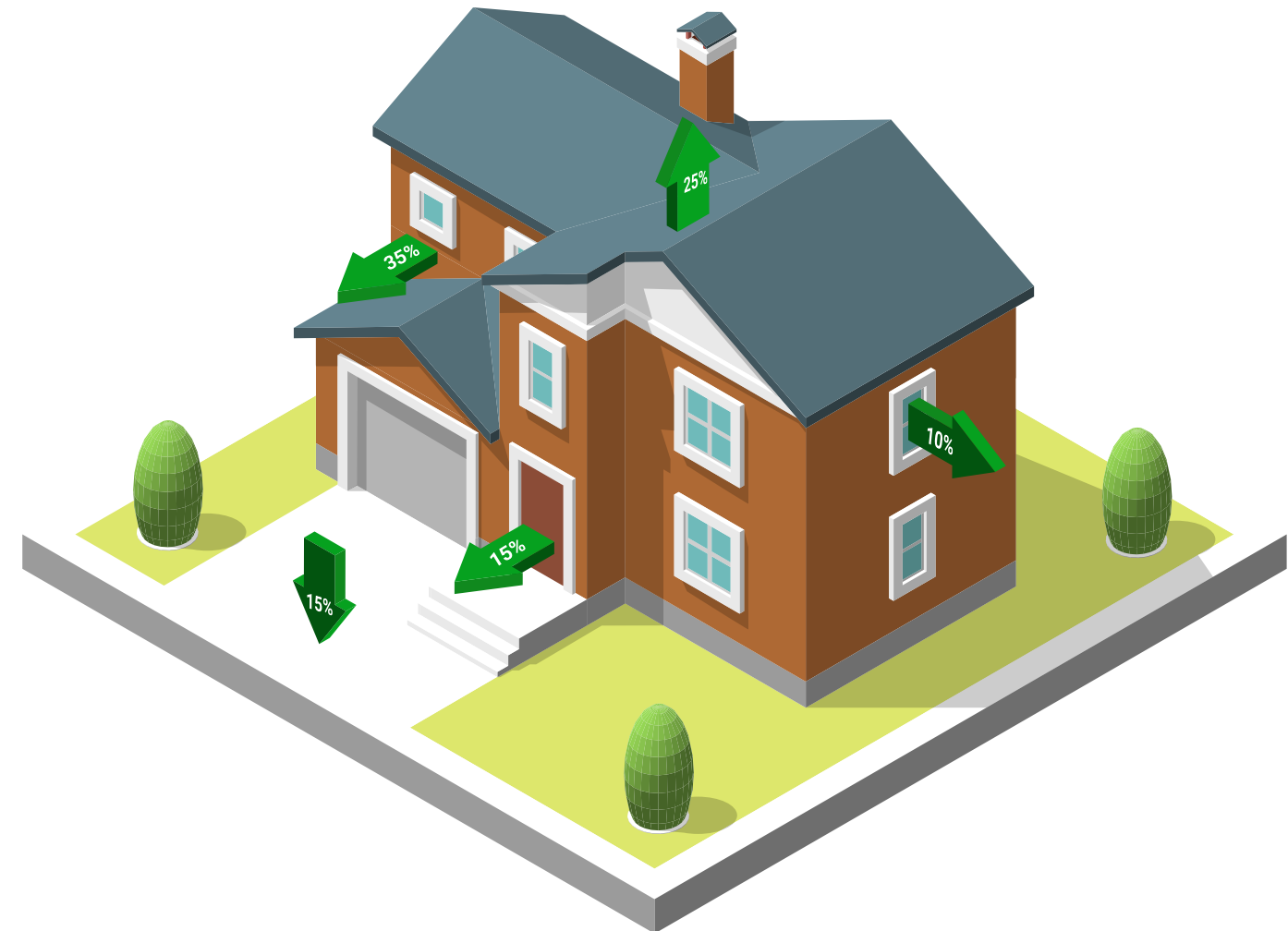
Figure 6.2: Direction and approximate percentage of loss, non-energy efficient private house
