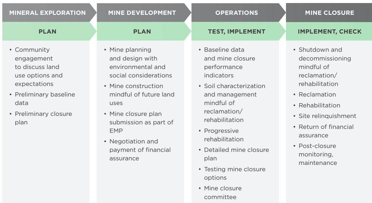
FIGURE 9. MINE CLOSURE PROCESS THROUGHOUT THE LIFE OF A MINE
