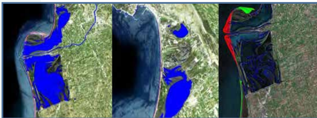
Figure 33. Drini i Lezhës River. Coastline changes and sea erosion for the period 1971 – 1986 – 2005 (left to right). (red - erosion, green - sedimentation)
