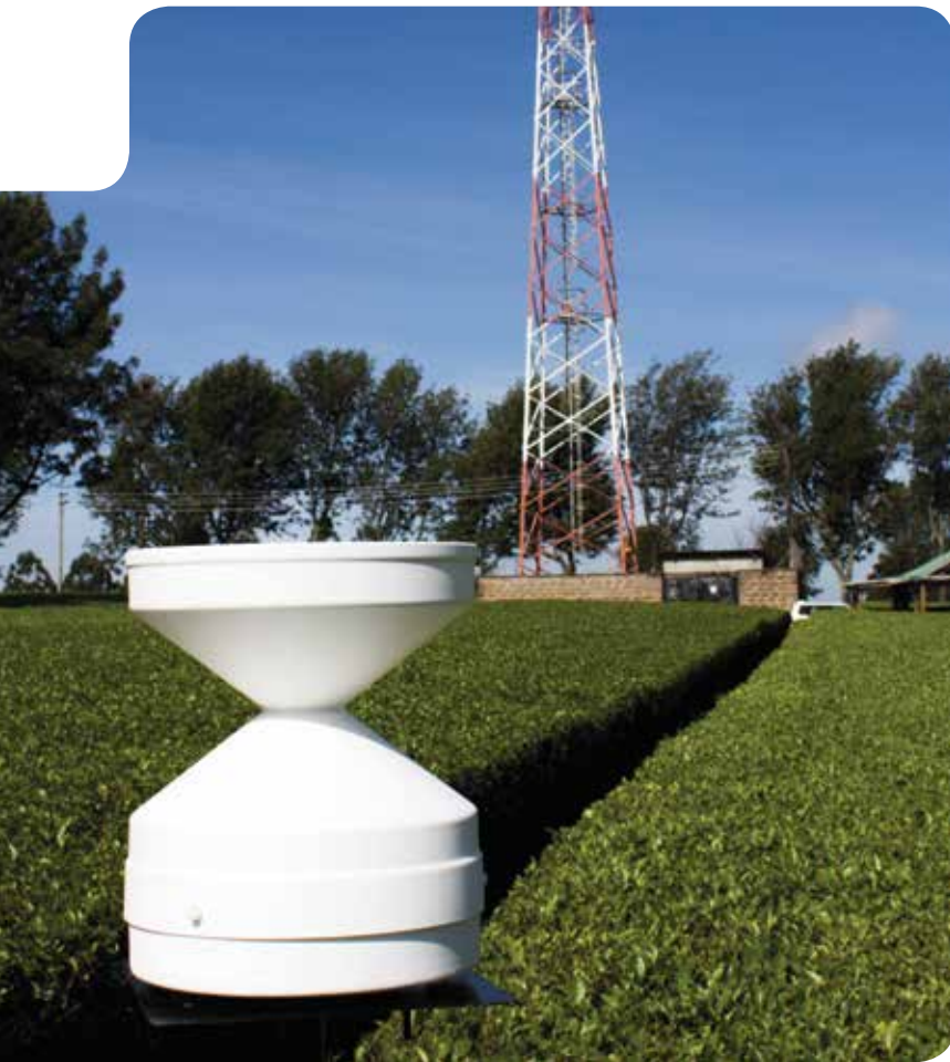
CELL-TOWER SITES CAN BE USED TO POSITION METEOROLOGICAL EQUIPMENT, EITHER ON THE TOWER, SUCH AS AN AUTOMATIC WEATHER STATION AND/OR A LIGHTNING LOCATING SENSOR, OR ADJACENT TO IT, SUCH AS THE RAIN GAUGE SHOWN HERE. THE CELL NETWORK CAN ALSO BE LEVERAGED TO DISTRIBUTE EARLY WARNINGS AND CLIMATE INFORMATION. PHOTO BY JOOST HOEDJES.
