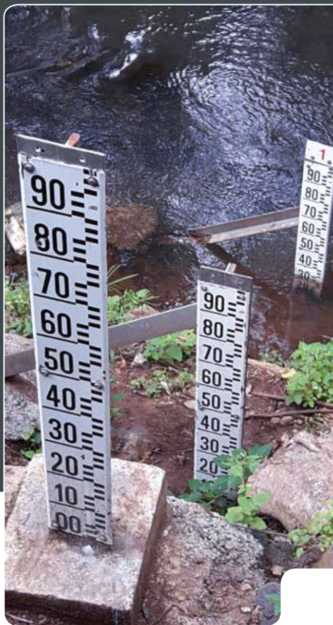
A SERIES OF STAFF GAUGES ARE USED TO MANUALLY OBSERVE RIVER LEVELS.
