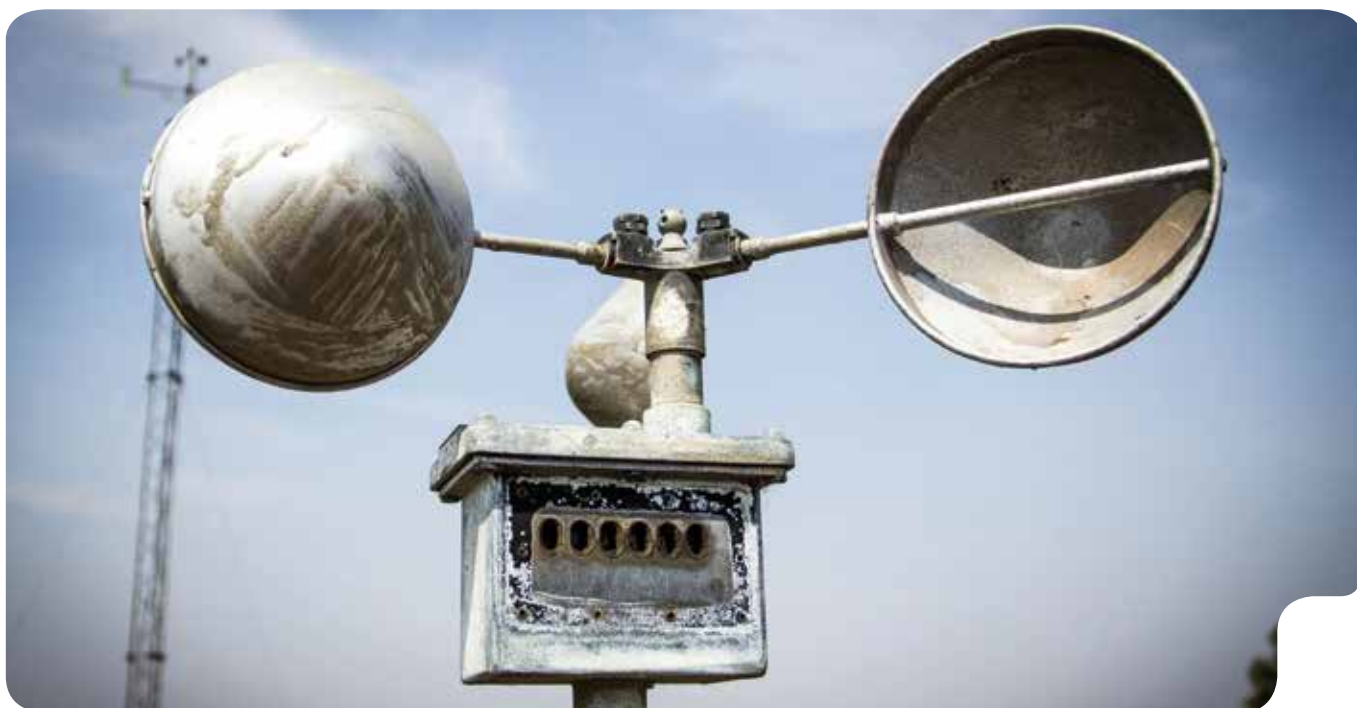
AS EVIDENCED BY THIS BROKEN ANEMOMETER, EVEN WHEN WEATHER AND CLIMATE MONITORING SYSTEMS HAVE BEEN PROPERLY DEPLOYED, SECURITY AND MAINTENANCE ARE ONGOING CHALLENGES. PHOTO BY JOOST HOEDJES.
