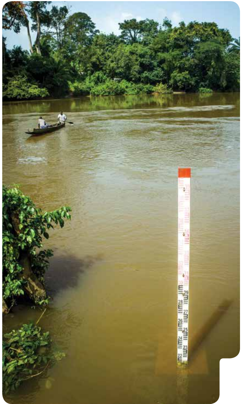
A TRADITIONAL RIVER-LEVEL GAUGE IN LIBERIA. PHOTO BY JOOST HOEDJES.
