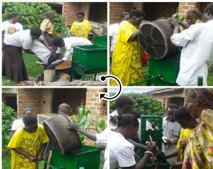
The Green Charcoal Sisters of Mubende district get started on the four-step process of making a new set of briquettes by preparing charcoal dust made from maize cobs before using clay soil to bind it into the “green charcoal” which is packed and sold within their community. The project supports both men and women to reduce on deforestation through improved charcoal production.
