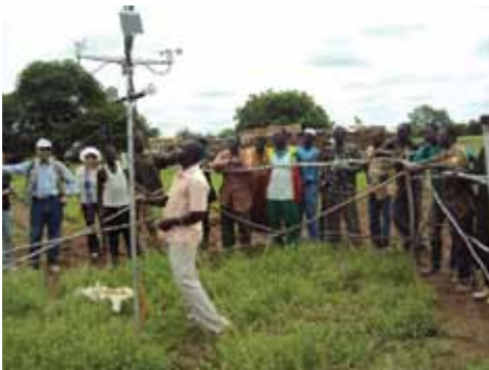
Automated weather stations, like this one being erected in Burkina Faso, have enabled countries to create more accurate and detailed forecasts and projects and to use these for short- and long-term planning needs.
