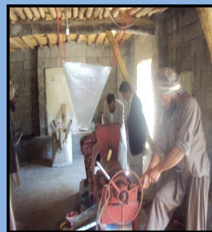
Figure 5: Operating Oil Expeller with electricity from NABDP's MHP in Dahan-a-Jamshad (Photo Credit: NaimatullahZafary)
