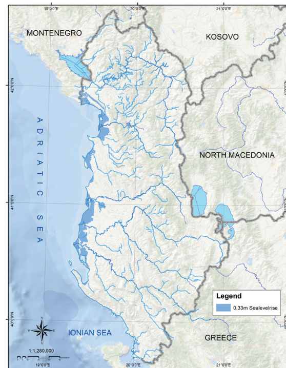
Figure 17. Coastal Zones that are likely to be flooded with 0.33m sea level rise
