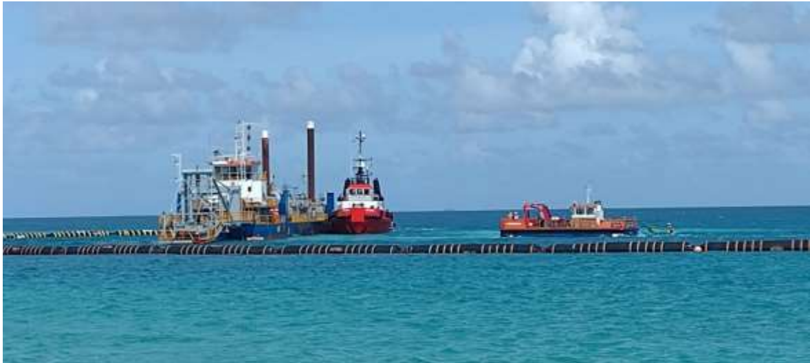
Figure 14: Example of suction dredge with dredge pipe off stern. Photo: P.Hawes
