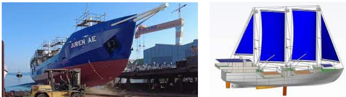
Figure 17. Example of hybrid vessel for Marshall Islands build in South Korea with wind-powered solution. Photo from Marshall Islands to get wind-powered solution to help decouple from international bunker prices | TradeWinds (tradewindsnews.com) and Concept Design example from Designing Wind Assisted Commercial Cargo Vessels > CAESES .
