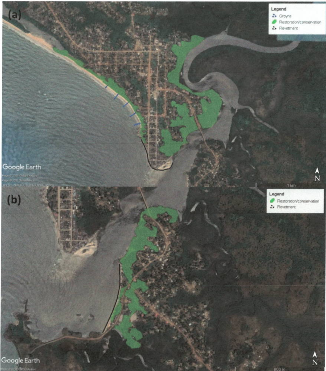
Figure 18. Proposed placement of the engineered and nature-based adaptation measures in the key sites of: (a) Downtown-Mississippi; and (b) Sebeh in Greenville. Diagrams of the placement of interventions in the remaining sites can be found in Annex 13d: Adaptation Options Report.
