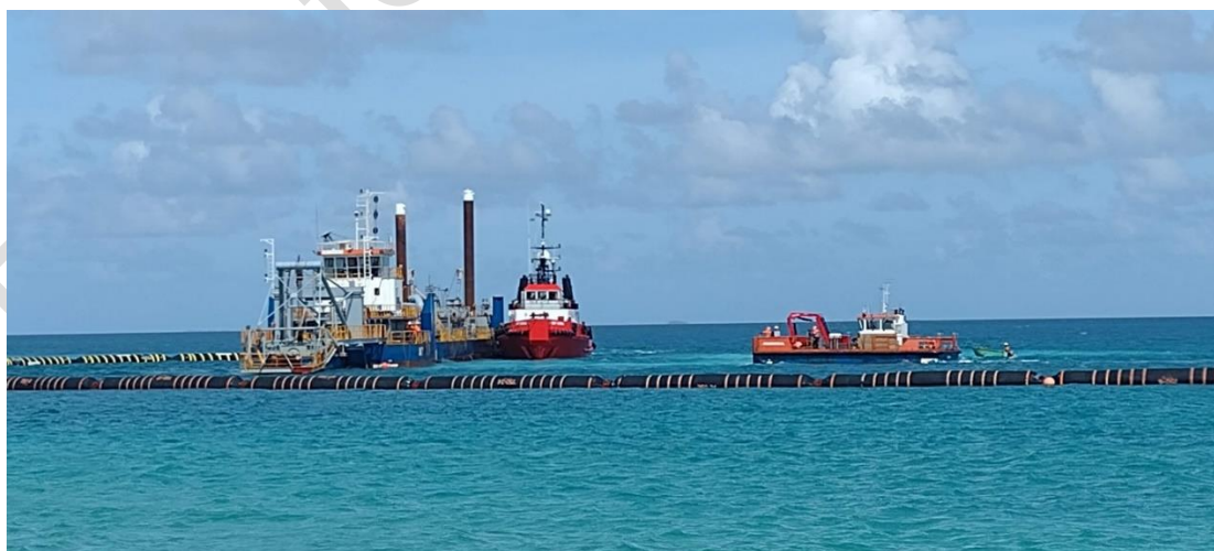
Figure 14: Example of suction dredge with dredge pipe off stern. Photo credit: P.Hawes
