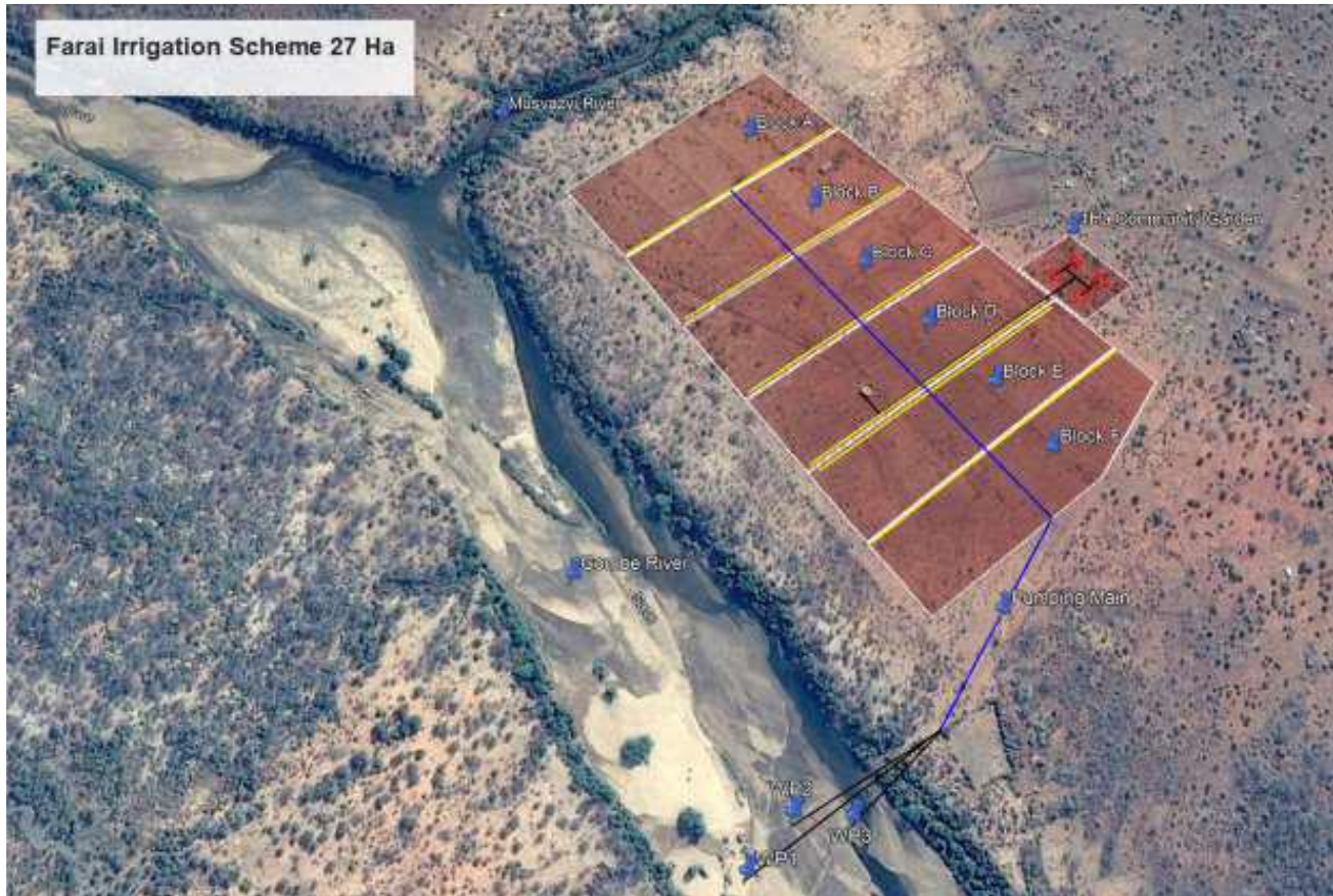
Figure 8: Configuration of Farai irrigation scheme
