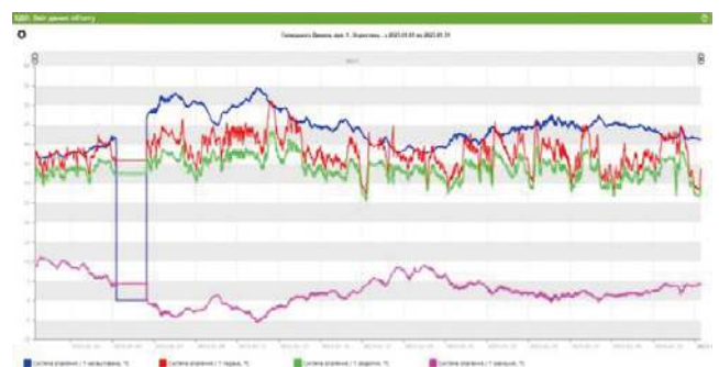
Picture 41. Weather-dependent heat carrier temperature regulation
