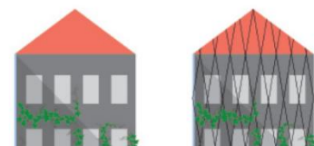
Graphic 6: Ground Based green walls. https://efb-greenroof.eu/green-wall-basics/
