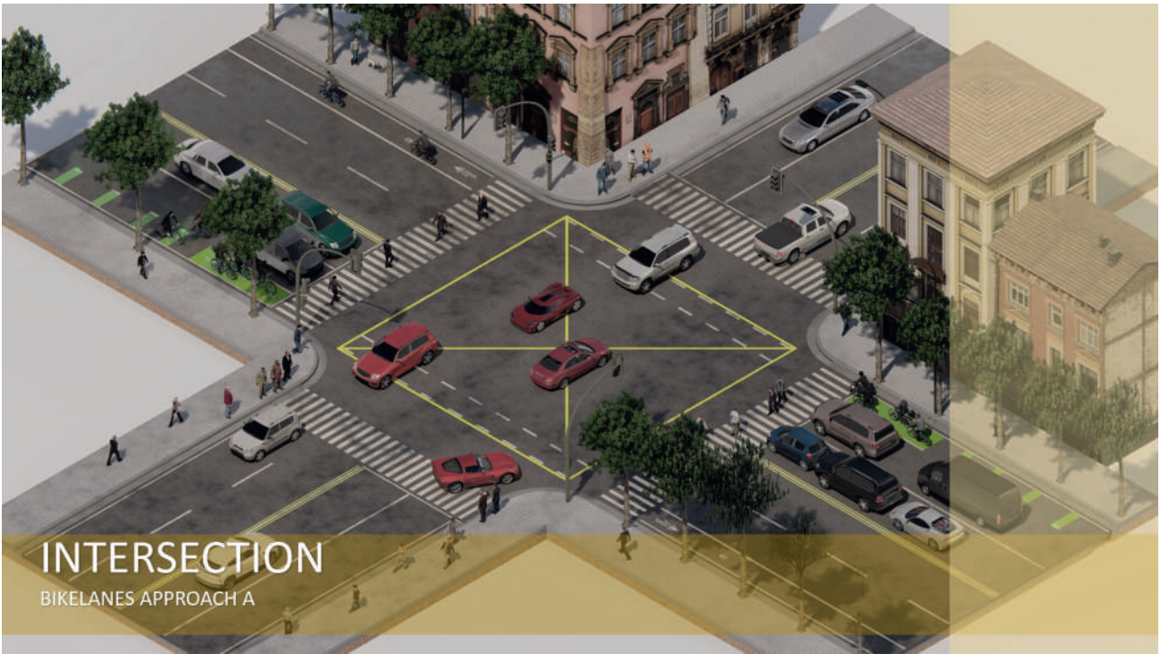
FIGURE 3.49 BIKE LANE INTERSECTION APPROACH "A"
