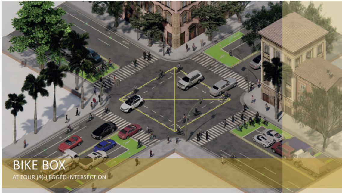
FIGURE 3.55 BIKE BOXES AT A 4-LEG INTERSECTION
