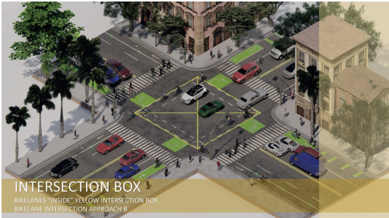
FIGURE 3.47 BIKE LANES INSIDE YELLOW INTERSECTION BOX
