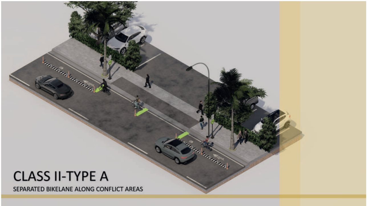
FIGURE 3.37 CLASS II-TYPE A: SEPARATED BIKE LANE ALONG CONFLICT AREAS USING BOLLARDS AND PRE-CAST CONCRETE DELINEATORS
