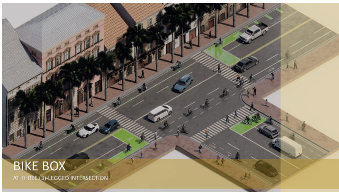
FIGURE 3.56 BIKE BOXES AT A 3-LEG INTERSECTION
