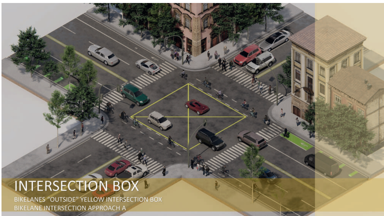
FIGURE 3.48 BIKE LANES OUTSIDE YELLOW INTERSECTION BOX
