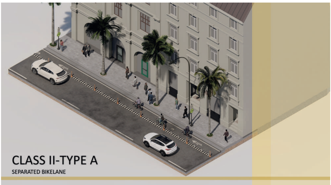
FIGURE 3.36 CLASS II-TYPE A: SEPARATED BIKE LANE USING BOLLARDS AND PRE-CAST CONCRETE DELINEATORS
