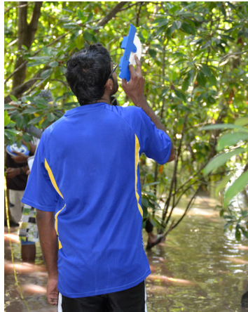
Figure 6: Measuring height of tree using Clinometer.
