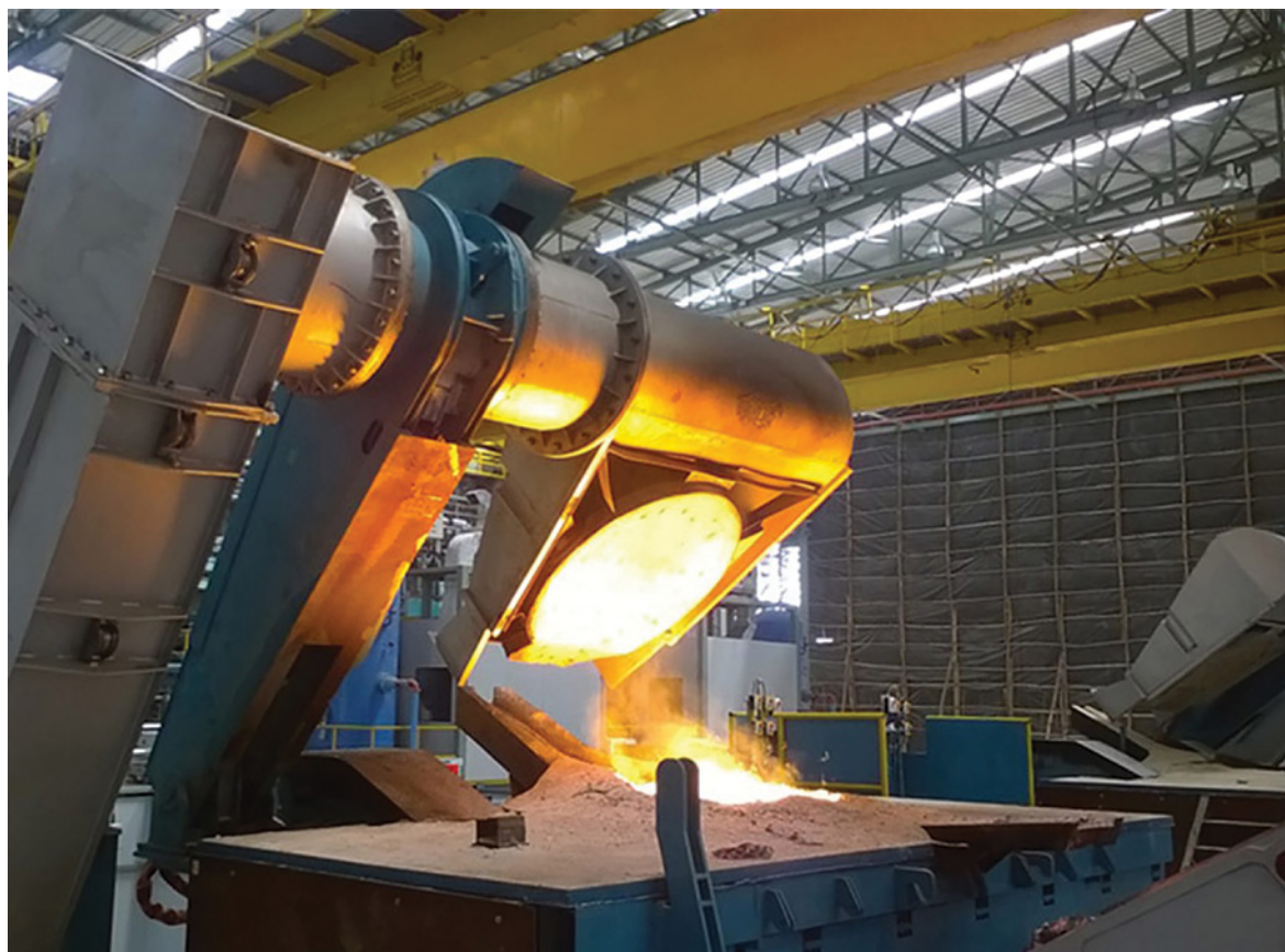
Induction furnace lid mechanism
