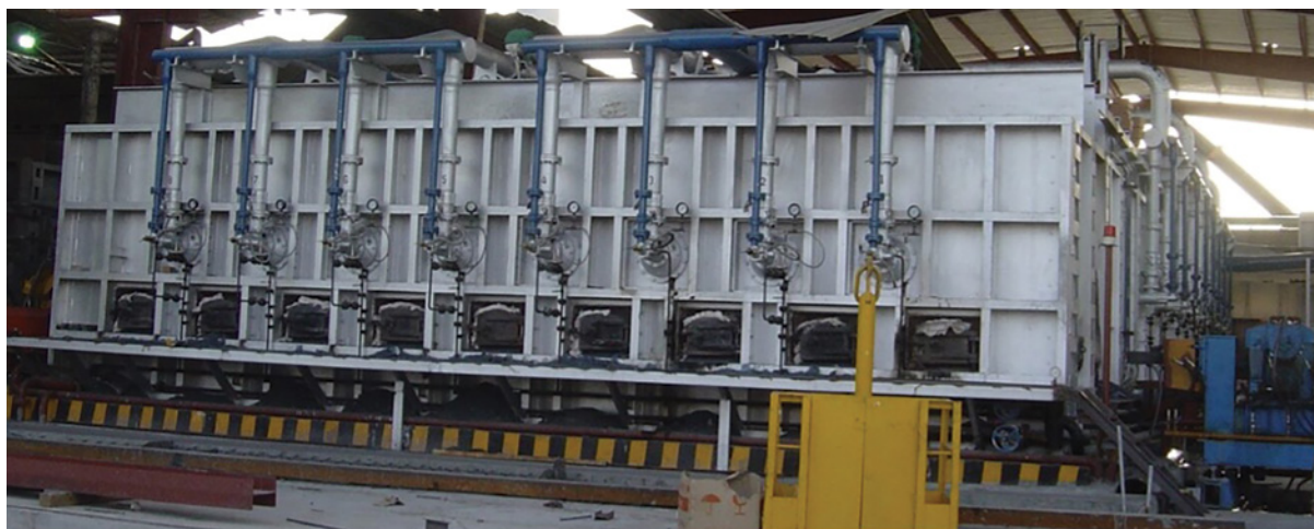
Energy efficient re-heating furnace
