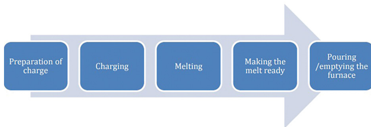
Induction furnace process
