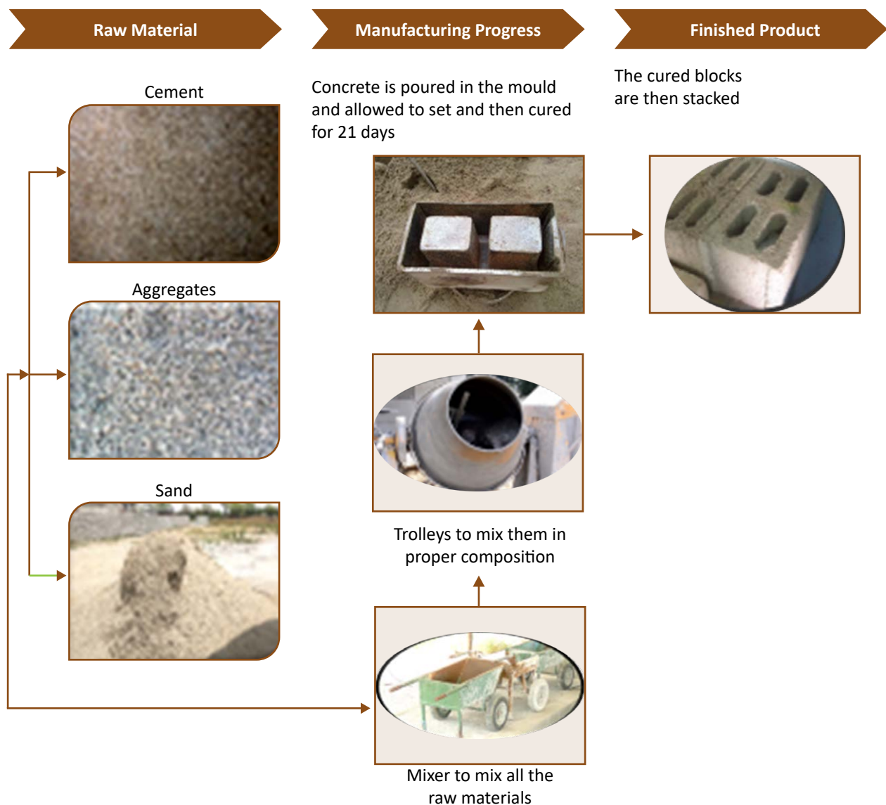
Figure 9: Manufacturing process for precast hollow blocks
