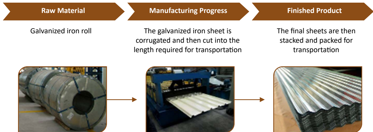
Figure 22: Manufacturing process for CGI sheets
