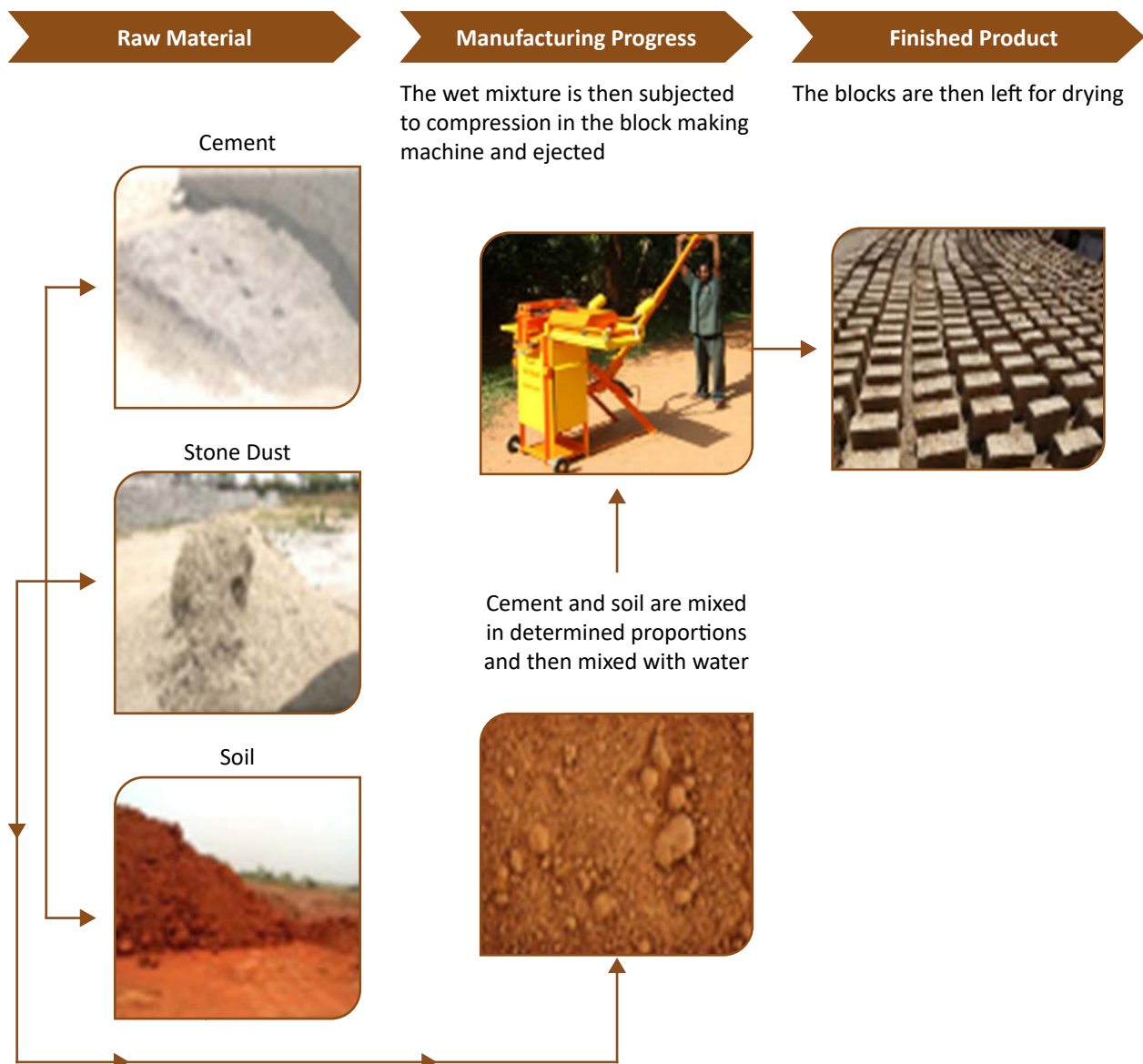
Figure 10: Manufacturing process for CSEBs
