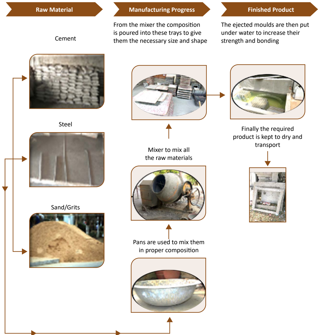
Figure17: Manufacturing process of ferro cement door and window frames
