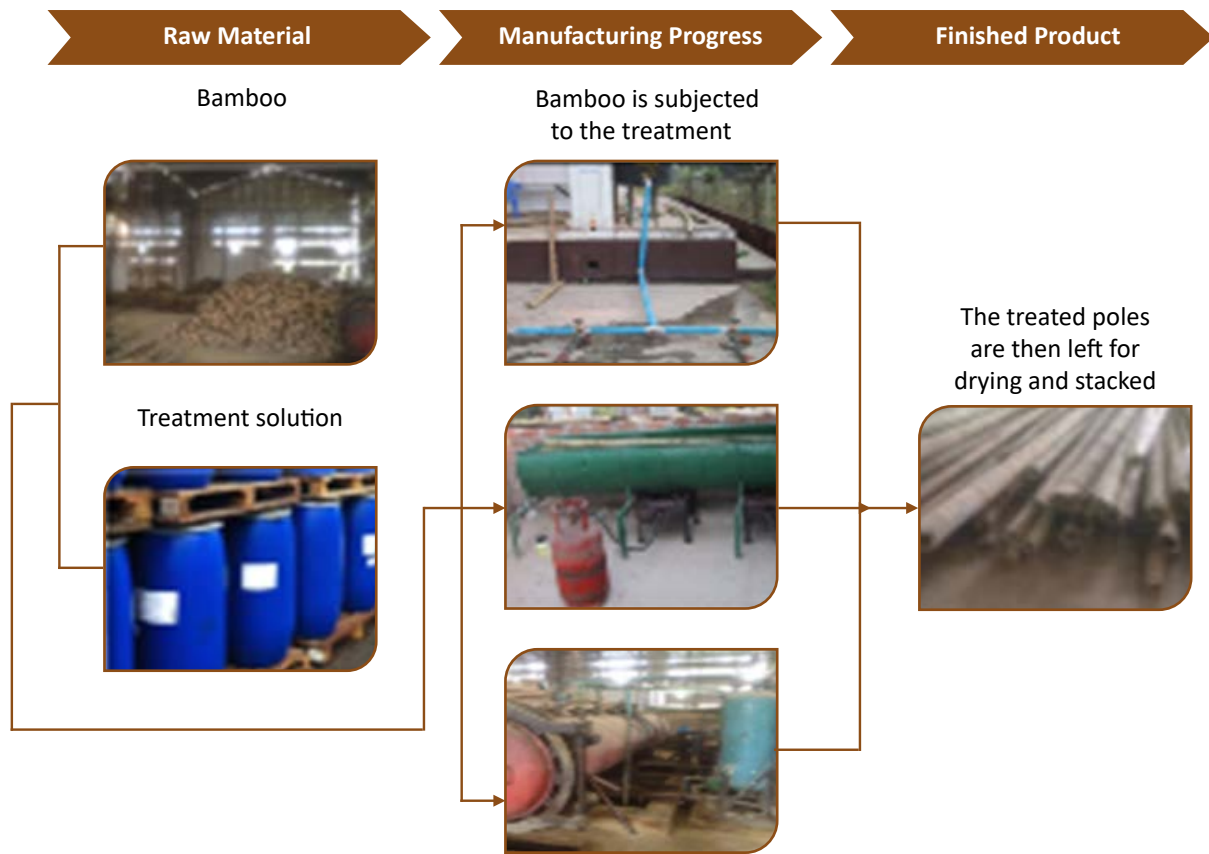
Figure 4: Treatment process for bamboo
