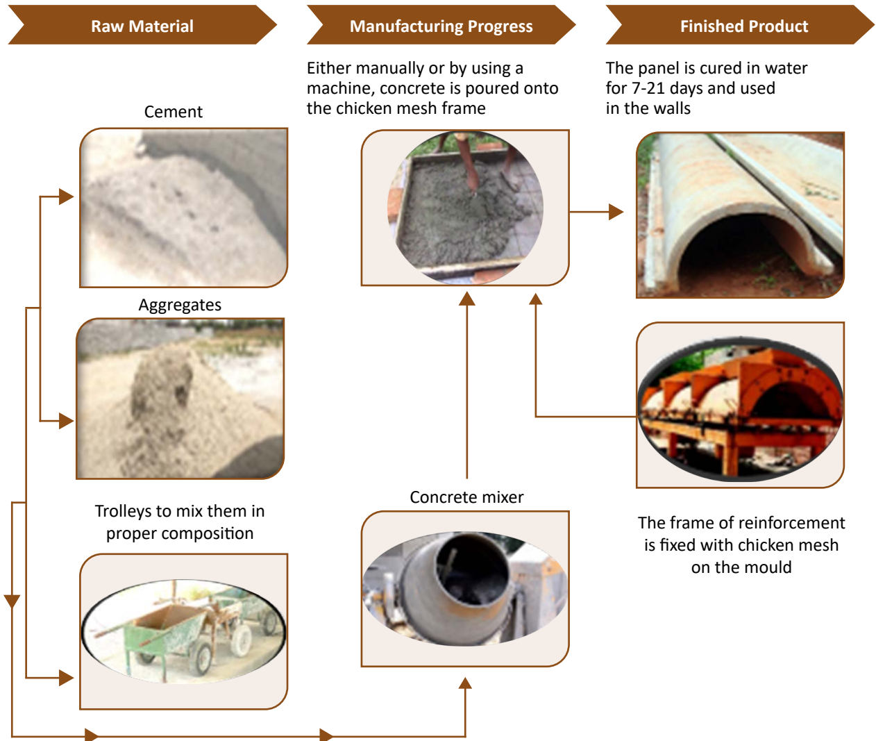
Figure 20: Manufacturing process of ferro cement roofing channel
