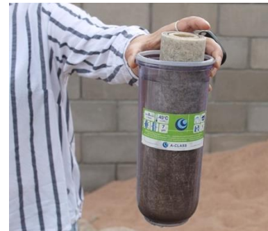
Dirty water filter from the village of Kadji Sai
