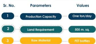
Table 18: Parameters of Recycling Unit (Shredder)
