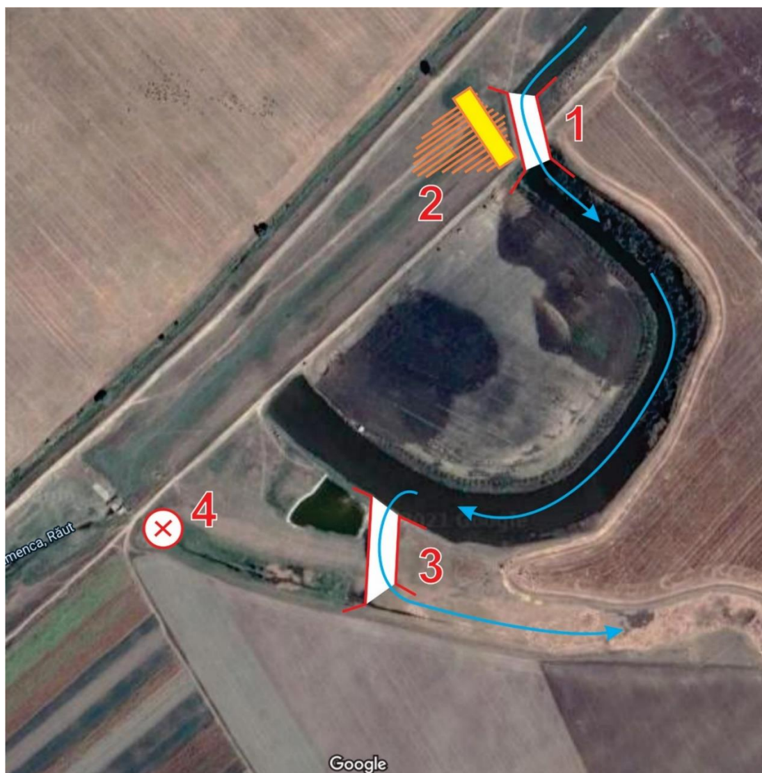
Fig. 9. Scheme of location of the hydrotechnical constructions, according to scenario 2. The arrows show the direction of waterflow after the constructions are made
