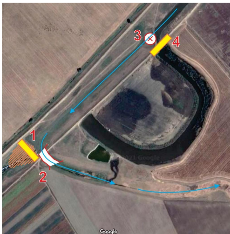
Fig. 10. Scheme of location of the hydrotechnical constructions, according to scenario 3. The arrows show the direction of waterflow after the constructions are made
