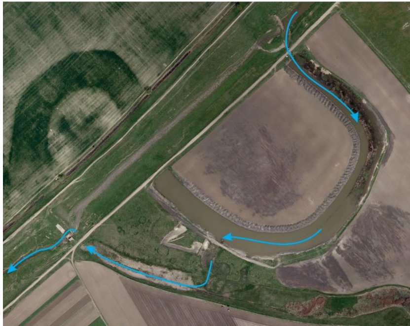
Fig. 7. Unauthorized hydrotechnical construction (reservoir) (orthophoto 2016). The arrows show the direction of waterflow nowadays
