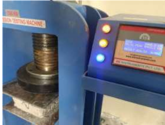
Fig: Compressive strength testing of pavement tiles and interlock bricks
