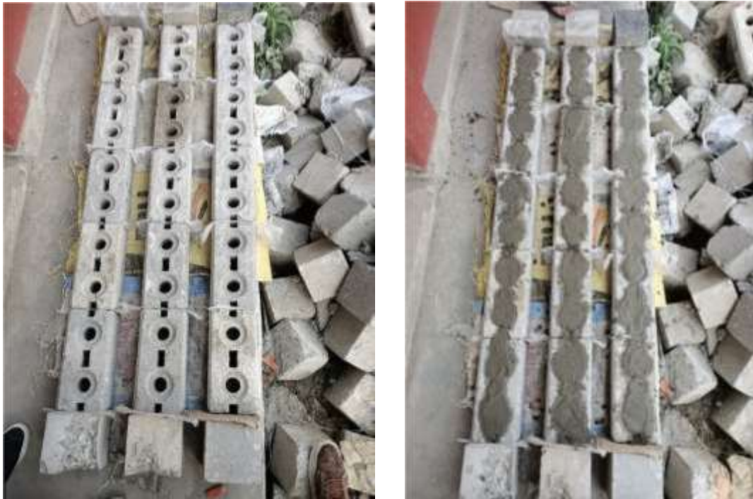
Fig: Sample preparation of solid bricks for lab test
