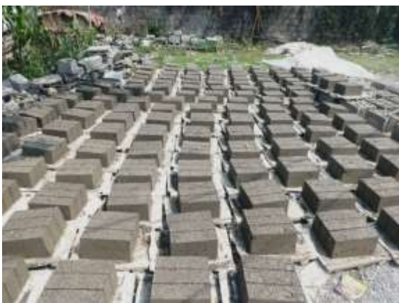
Fig: Mass production of plastic mixed solid bricks
