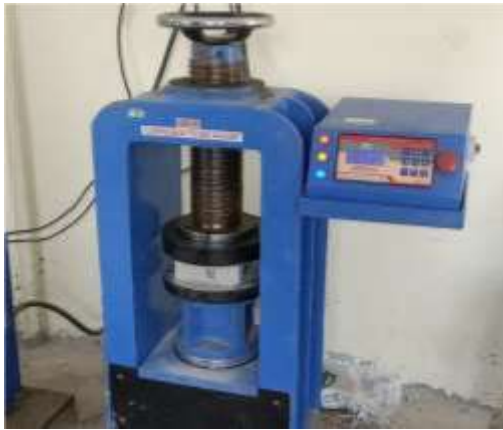
Fig: Compressive strength testing of pavement tiles and interlock bricks
