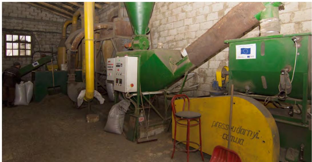
▲ Ukrainian briquettes production line, with a production capacity of 400 kg/h
