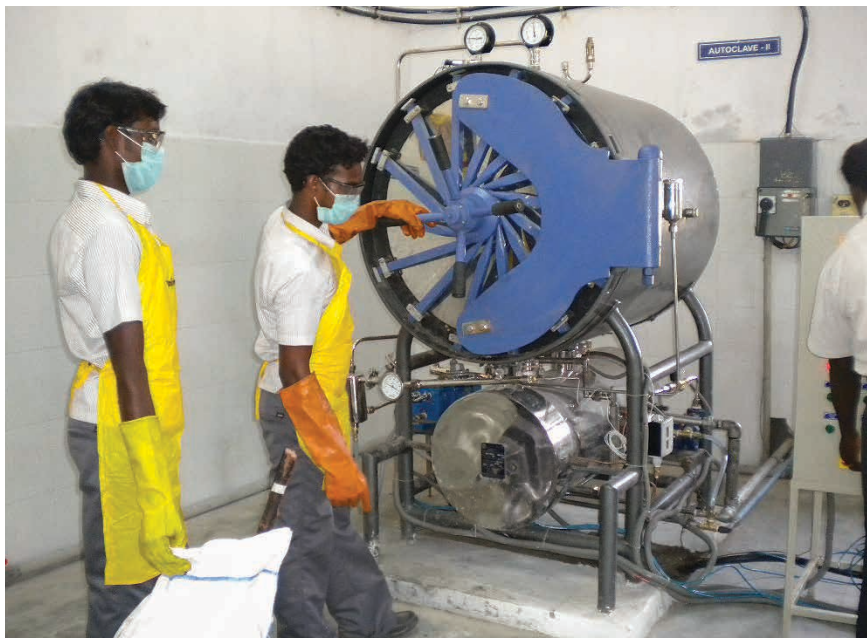
UNDP-GEF project installed autoclave technology at a biomedical waste treatment plant in Chennai, India GJ Multiclave plant, Chennai, Tamil Nadu, India; 2012
