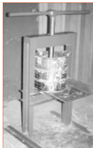
The improved bridge press reduces fuel and water use, as well as exposure to smoke and heat.
